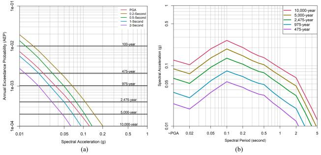
Figure 3. 5%-damped, (a) mean hazard curve, (b) mean horizontal acceleration uniform hazard response spectra.
