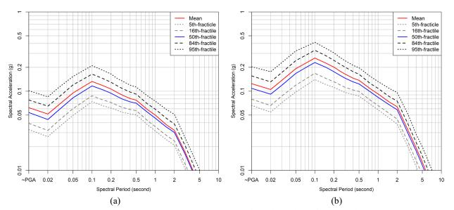
Figure 5. 5%-damped, horizontal acceleration UHRS of the mean,  $5^{th}$ -,  $16^{th}$ -,  $50^{th}$ -,  $84^{th}$ -, and  $95^{th}$ -fractiles for (a) 1 in 2,475 AEP, (b) 1 in 10,000 AEP.
