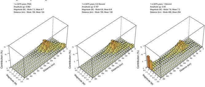
Figure 4. Magnitude-distance deaggregation for the 1 in 2,475 AEP hazard at selected spectral periods.
