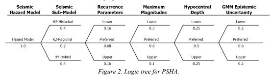
The minimum earthquake magnitude used in the PSHA is M4.8 as in Halchuk et al. [1]. Earthquakes with lower magnitudes are generally considered incapable of developing long-duration ground motions and are, therefore, of limited engineering significance to modern engineered structures.
